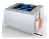
AtmoMix<sup>®</sup> Gas mixer for 2 or 3 gases, with either preset or user adjustable gas mix ratios
